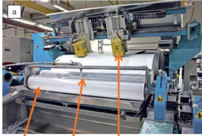
Pick-up roll Nip feeder Gauge control
